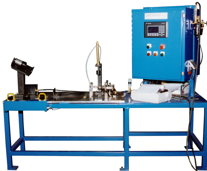
High Volume Mass Flow Leak Test and Weld Leak Repair Station
