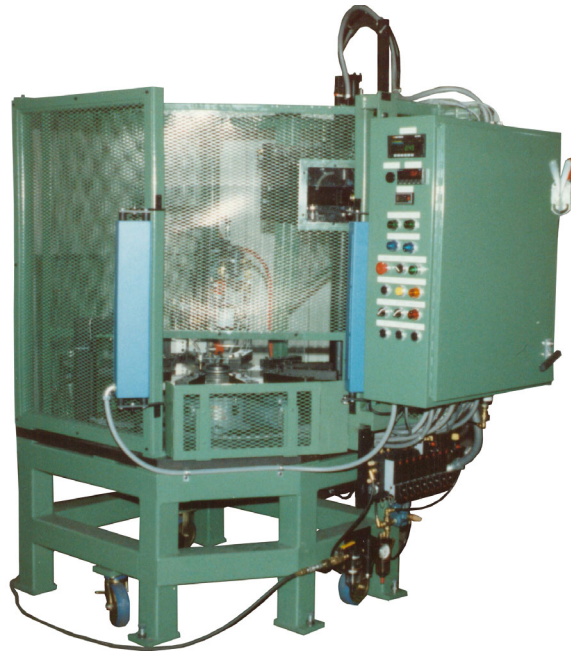
24 Station High Production Dial Table Nitrogen Mass Flow Leak Test Machine
