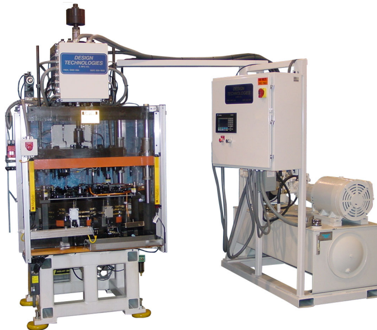
4 Post Hydraulic Broaching Die Set Press with 12 Position Dial Table
